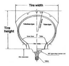
The other series of numbers and letters, MT90 16, represents the same tire size, but it's expressed in an alphabetical code. M means the tire is designated for motorcycle use, T is the tire width code, 90 is the aspect ratio and 16 is the rim diameter.
