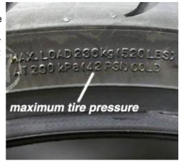
wear. If in doubt, either consult your owner's manual, contact your local dealer, or go to the tire manufacturer's website. Most include the recommended pressure for each motorcycle, along with other tire options. And be sure to measure pressure when the tire is cold. Measuring hot will skew the numbers.
